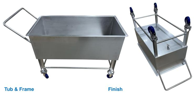
Formed 11 gauge / 304 stainless steel <u>(no hollow or tubular components)</u>. Inside dimensions of the tub are 48"L x 24"W x 17"D and features a Ø1" drainage hole with 1"L drainage tube.
